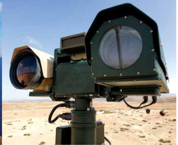
Units also offer a unique integration of electro – optical sensors and radar with a single telescopic mast to avoid any dead zone in observation area.
